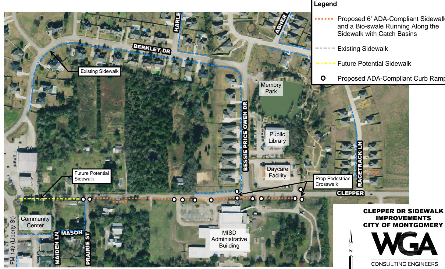
Proposed 6' ADA-Compliant Sidewalk and a Bio-swale Running Along the
