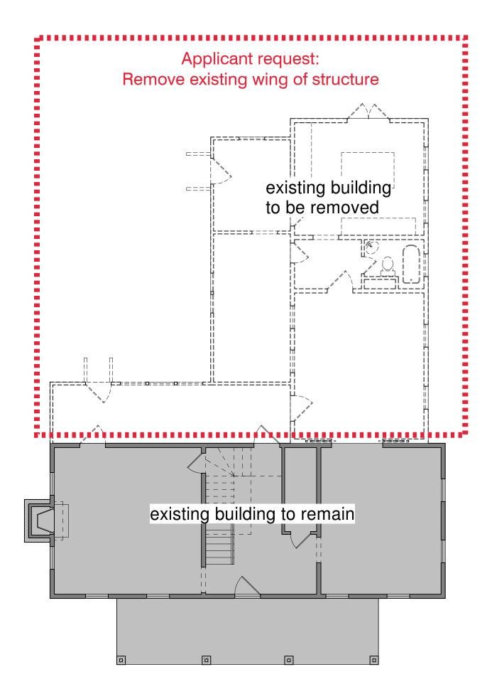
existing 1 st floor plan scale: 1/8" = 1'-0"
