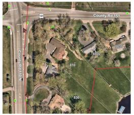
Figure 3. Storm sewer (green) and sanitary sewer (red) at CR 110 and CR 151
