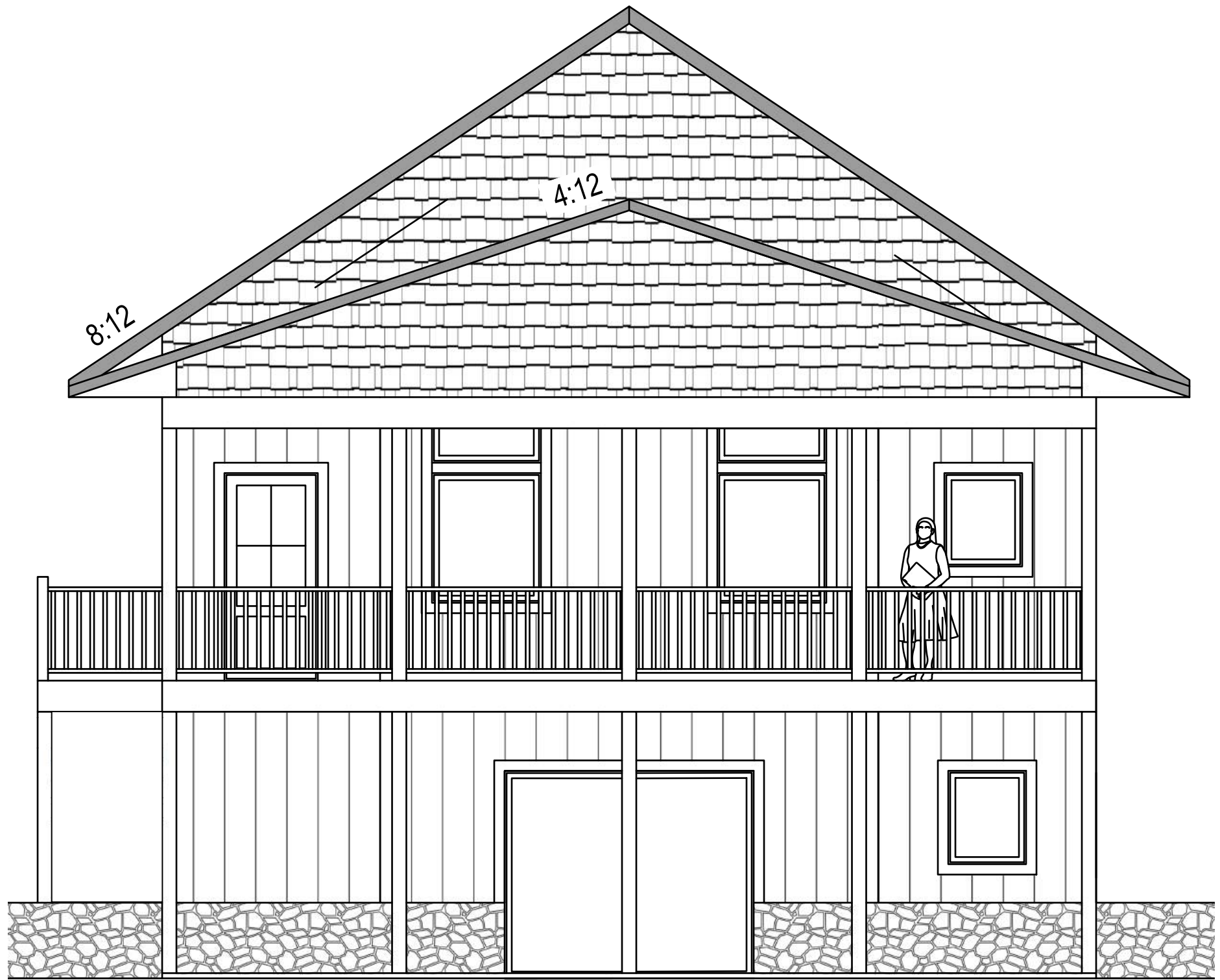
F WEST ELEVATION 1/4" = 1'-0"
