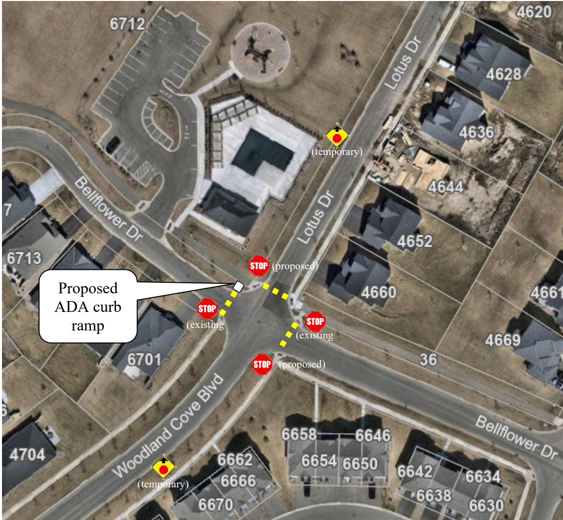
Figure 1. Proposed Installations at Woodland Cove Boulevard/Lotus Drive at Bellflower Drive: Stop Signs, Stop Ahead Signs (locations shown are approximate), Crosswalks (shown in yellow, will be painted white), and an ADA Curb Ramp
