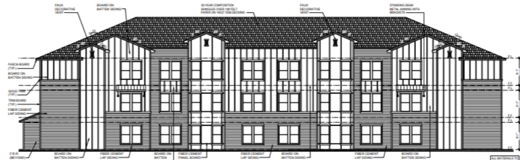
04 BUILDING 'B' - REAR ELEVATION SCALE: 1/8" = 1'-0" 1 RECD @ BLDG #2
