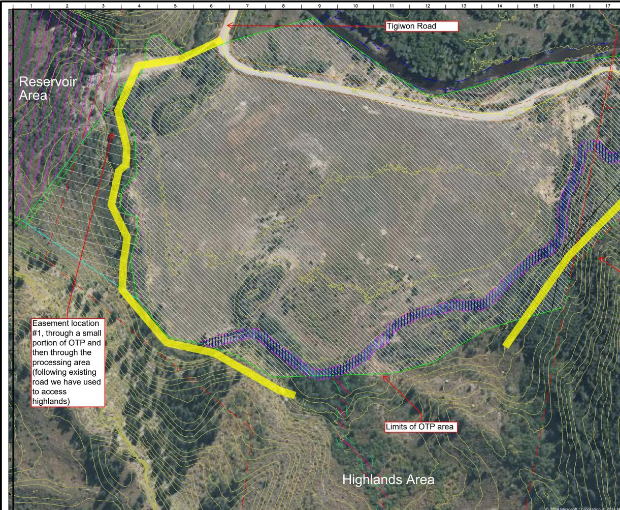
Easement location #2 (assume 100' wide easement), from the corner of Tigiwon road to Highlands, this road would require tree clearing and grading, but is outside the limits of the remediation area and could be maintained during reservoir construction. Proposed Easements to Highlands Minturn, CO
