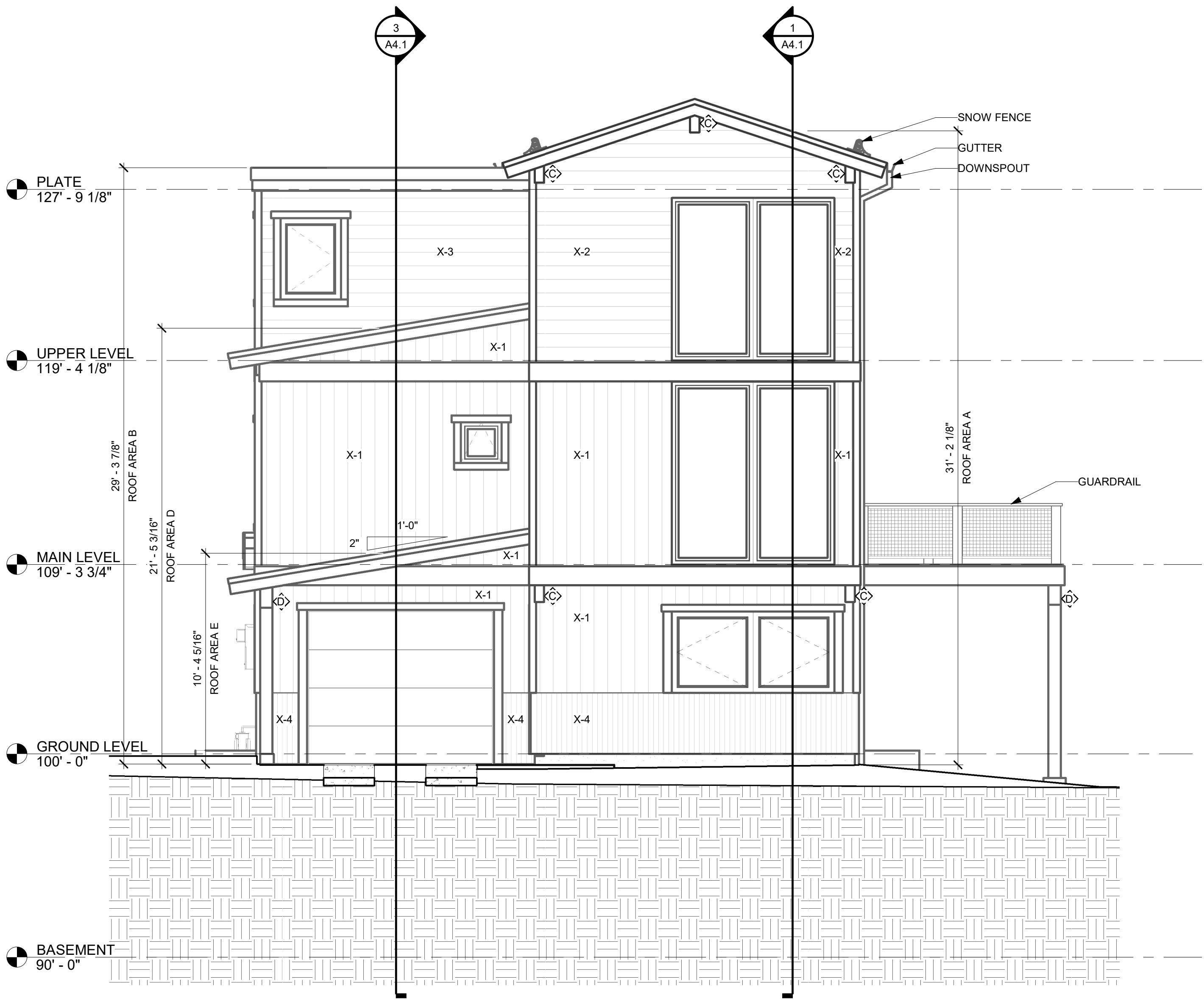
4 FRONT ELEVATION A3.1 1/4" = 1'-0"
