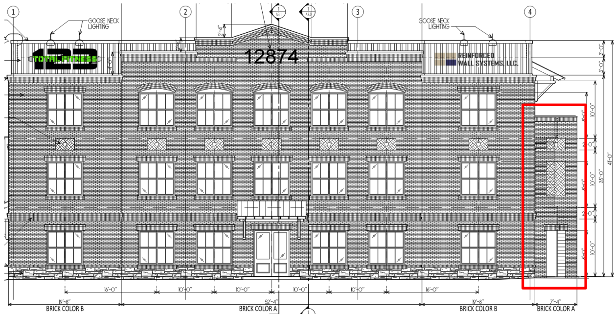
Drawing 2: Screen wall viewed from the North Elevation
