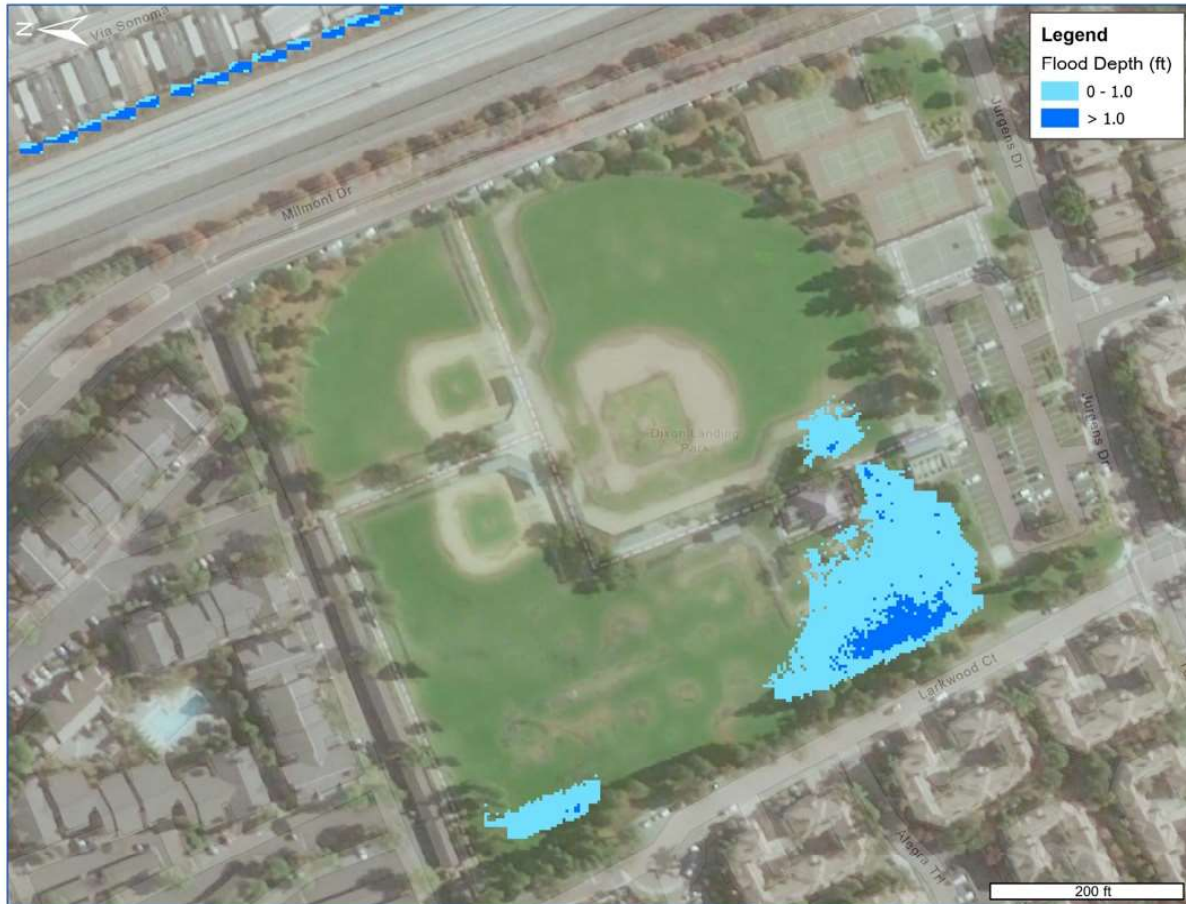
Figure 4-2: 10-year Ponding Adjacent to Jurgens Pump Station
