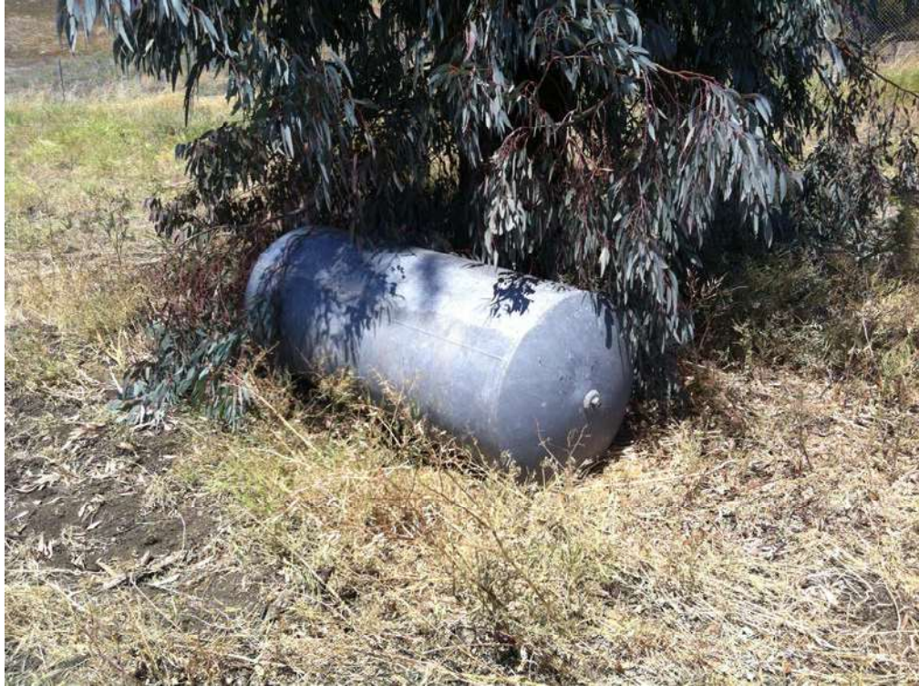
Photo 9: Abandoned aboveground storage tank that may have formerly been used for hot water storage. Tank located on east-central portion of the site. Photo taken in June 2015.
