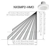
Sensor Lens Coverage and Detection Patterns When Mounted at 40ft and 45ft with Standard Lens
