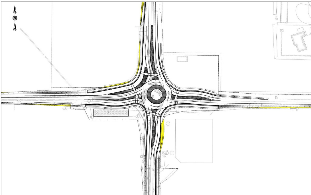
Figure 2. Roundabout with Bypass Layout
