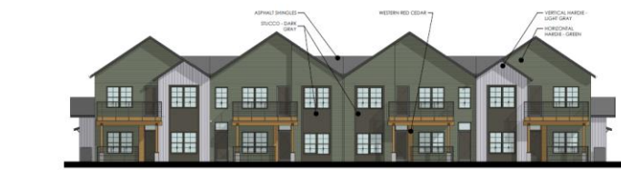
1 | FRONT ELEVATION - BUILDING 04
