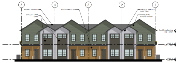
1 | FRONT ENTRY ELEVATION 13'0" x 17'0"
