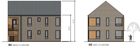
Boulder Flats Building Type B - Concept Elevations SCALE: 1/8" = 1'-0"
