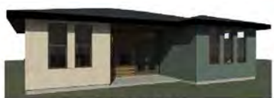
HIP ROOF - BACK VIEW
