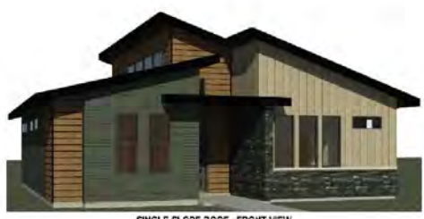
SINGLE SLOPE ROOF - FRONT VIEW
