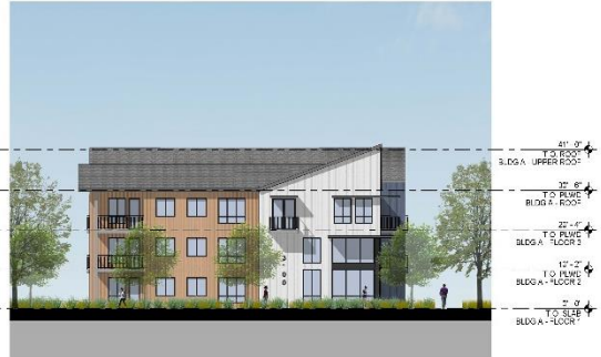
BUILDING A - WEST ELEVATION 3 1/16" = 1'-0"
