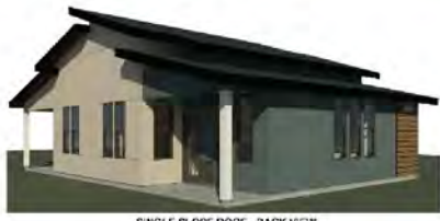
SINGLE SLOPE ROOF - BACK VIEW
