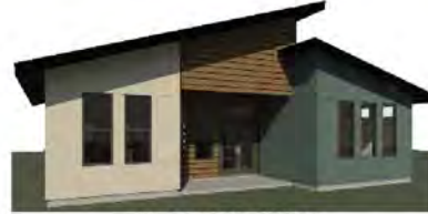
SINGLE SLOPE ROOF - BACK VIEW
