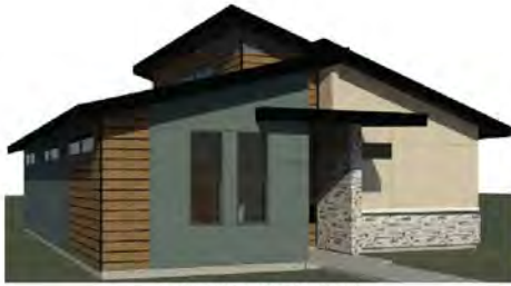
SINGLE SLOPE ROOF - FRONT VIEW
