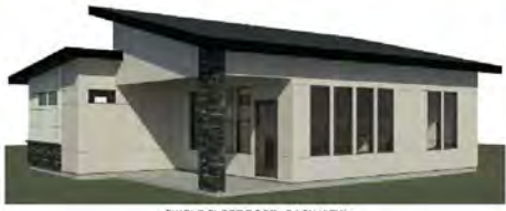
SINGLE SLOPE ROOF - BACK VIEW
