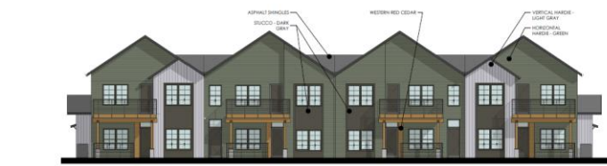
1 | FRONT ELEVATION - BUILDING 04
