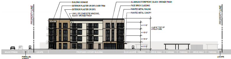
2. WEST (ENTRY DRIVE) ELEVATION
