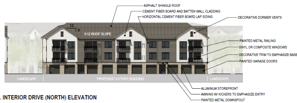
4. INTERIOR DRIVE (NORTH) ELEVATION
