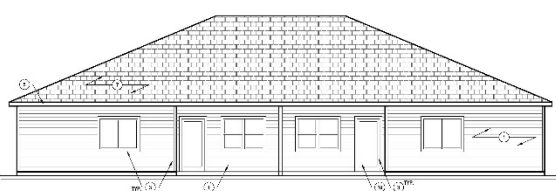
2B PATIO (REAR) ELEVATION - HIP ROOF OPTION SCALE: 3/8" = 1'-0"
