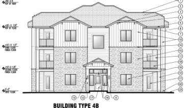
2 BUILDING TYPE 4B LEFT SIDE ELEVATION
