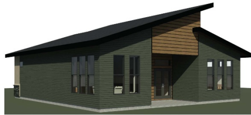
SINGLE SLOPE ROOF - BACK VIEW
