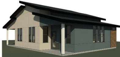
SINGLE SLOPE ROOF - BACK VIEW
