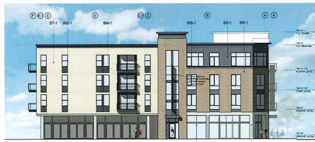
2 EAST ELEVATION - BLDG. B
