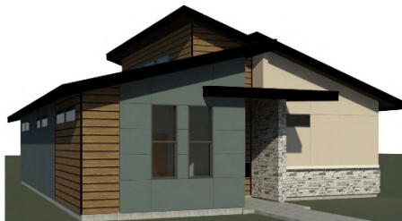
SINGLE SLOPE ROOF - FRONT VIEW
