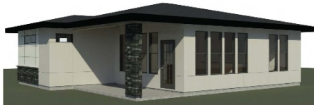
HIP ROOF - BACK VIEW
