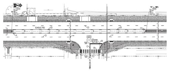
Design is planned to be complete by summer 2022. A landscape planting plan is being created for the basin adjacent to this project. Construction in 2024. Widen Eagle to 5 lanes with curb, gutter, sidewalk and a multi-use pathway. Includes a multi-lane roundabout at Eagle Rd and Taconic Dr. Here is the project website:
