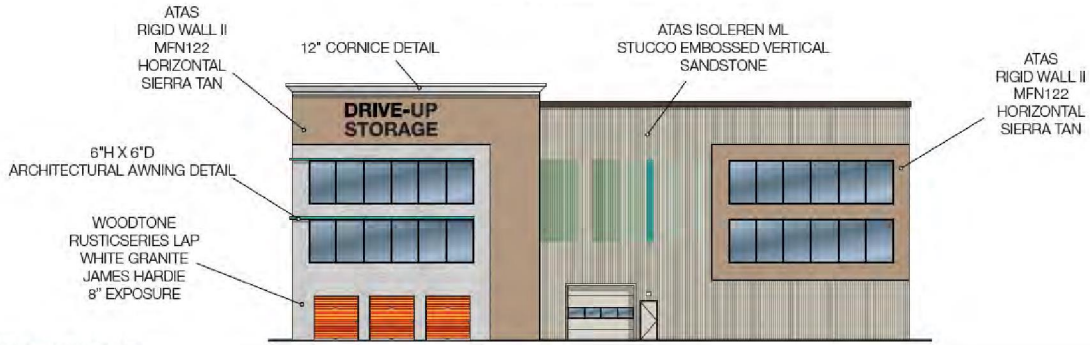
SOUTH ELEVATION: BUILDING B Scale: 1/16" = 1'
