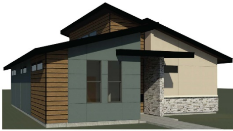
SINGLE SLOPE ROOF - FRONT VIEW
