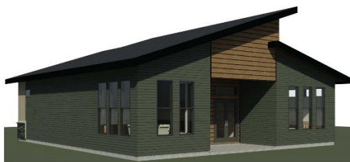
SINGLE SLOPE ROOF - BACK VIEW
