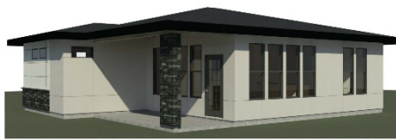
HIP ROOF - BACK VIEW
