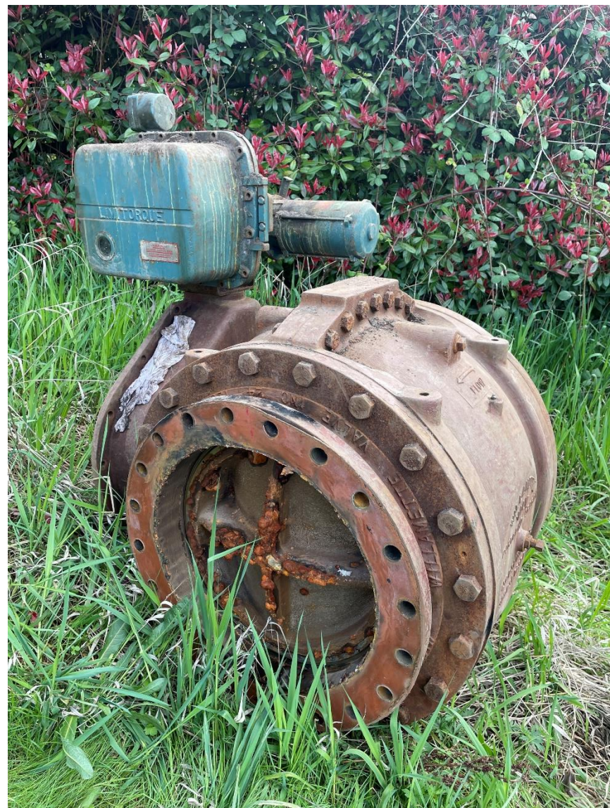
24-in ball valve that stuck closed
