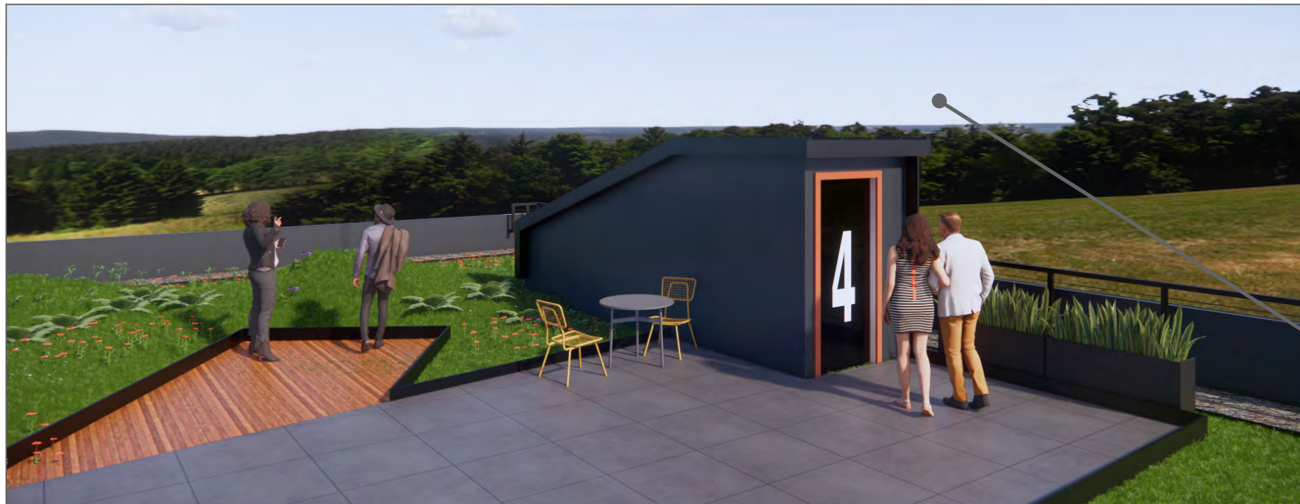
PROPOSED • EXTEND THE PARAPET TO 42" HIGH WITH A SIMPLE CLEAN PARAPET HANDRAIL. • PROVIDE A BARRIER AROUND THE DESIGNATED WALKWAYS AND INCORPORATE IT AS AN ARCHITECTURAL DETAIL AROUND NORTH SIDE OF DOG HOUSE. • ADDING PLANTERS AS AN ADDITION BARRIER ALONG THE DESIGNATED WALK WAYS.
