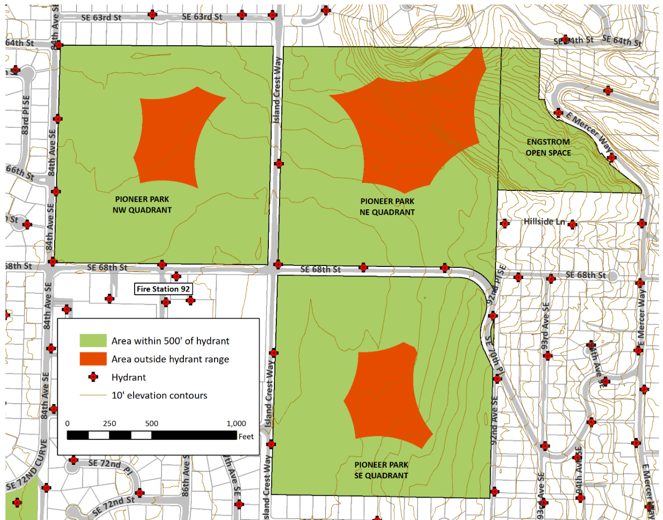
Figure 1: Map showing hydrant locations and coverage in Pioneer Park and Engstrom Open Space.
