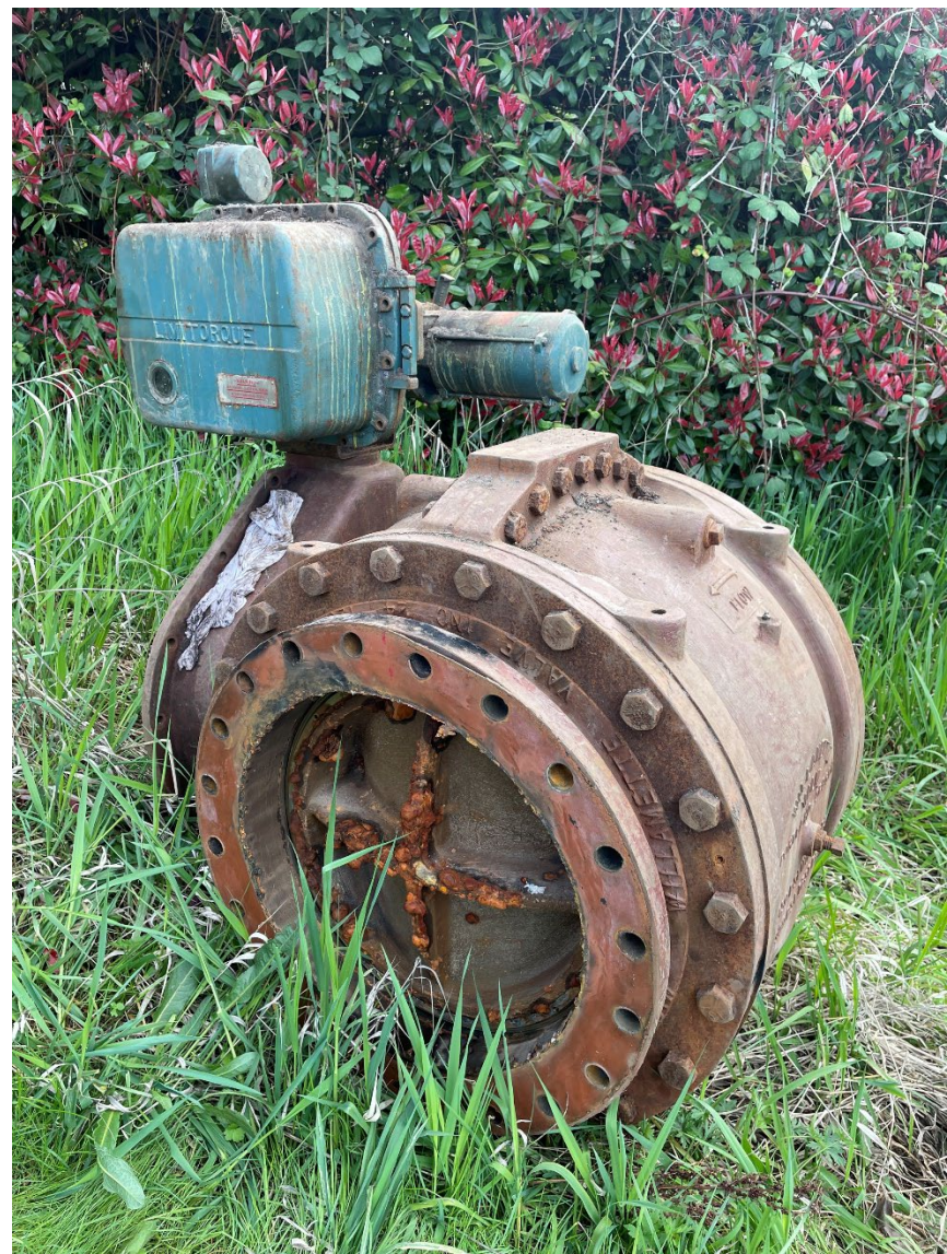
24-in ball valve that stuck closed
