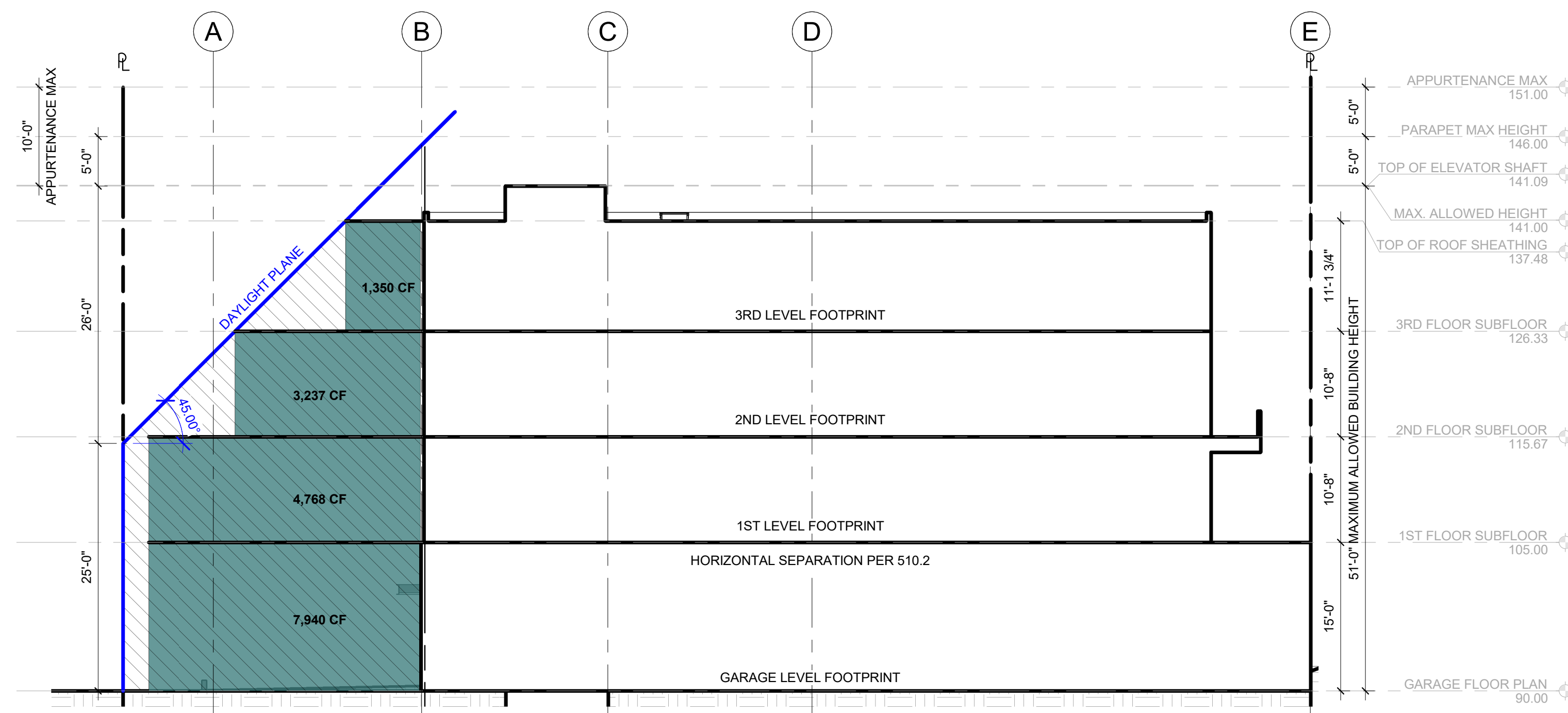
DAYLIGHT PLANE - CREDIT VOLUME 1" = 10'-0" 3
