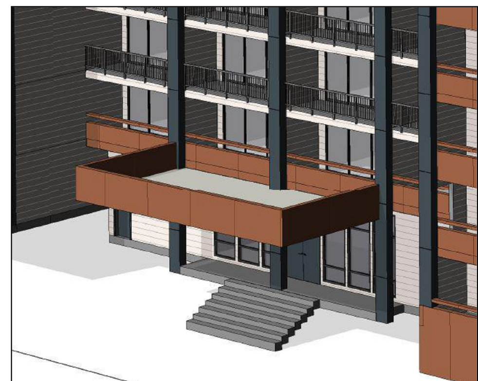
ORIGINAL ENTRY CANOPY WRAPPED IN TRESPA
