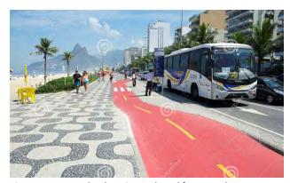
Figure 2. Example showing colored/textured pavement used to demarcate bike and pedestrian travel ways (Brazil)
