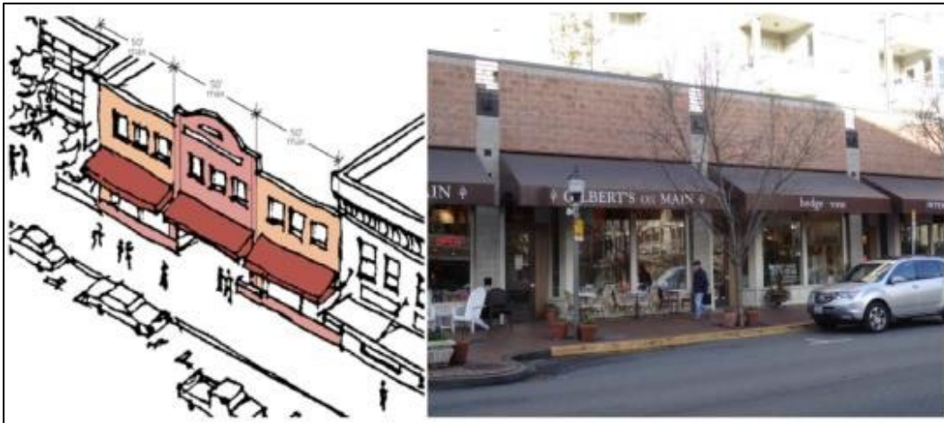
Figure 13 — Minor Facade Modulation Examples
