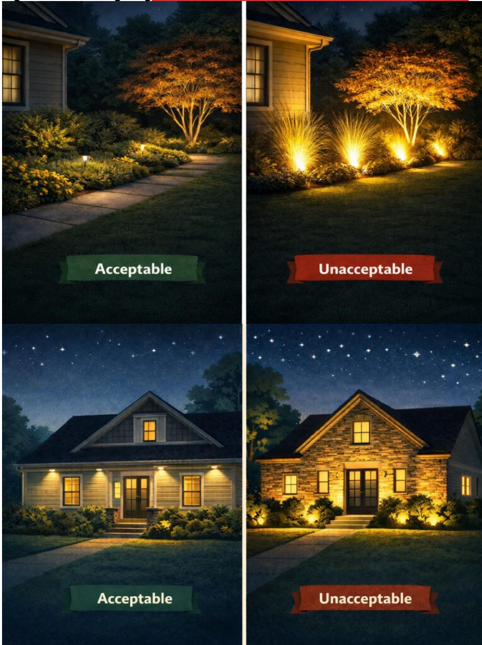
Figure 4: Accent Lighting: Shielded & Downcast vs. Unshielded & Upward Cast
