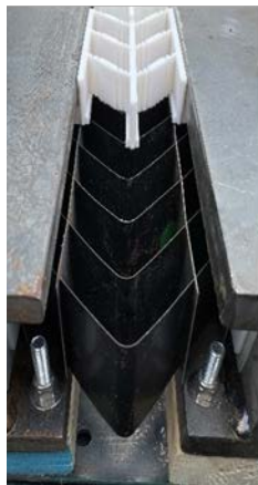
Figure 2-5. A) Set-up for static compression testing. B) Measured results from compression testing.
