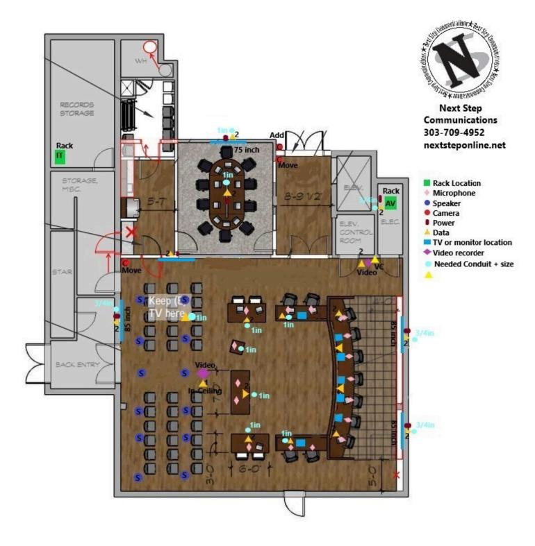
Layout with conduit sizes needed installed by the electrician for the TV and floor boxes
