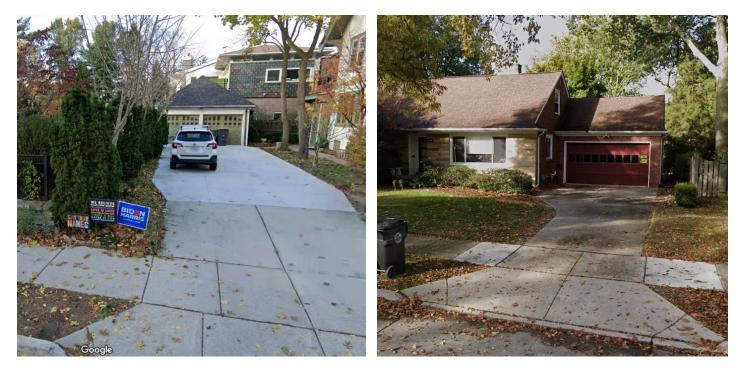
Both of these driveways have limited widths at the front property line, but taper/widen to a point approximately eighteen (18") inches beyond the outer edges of the garage door.
