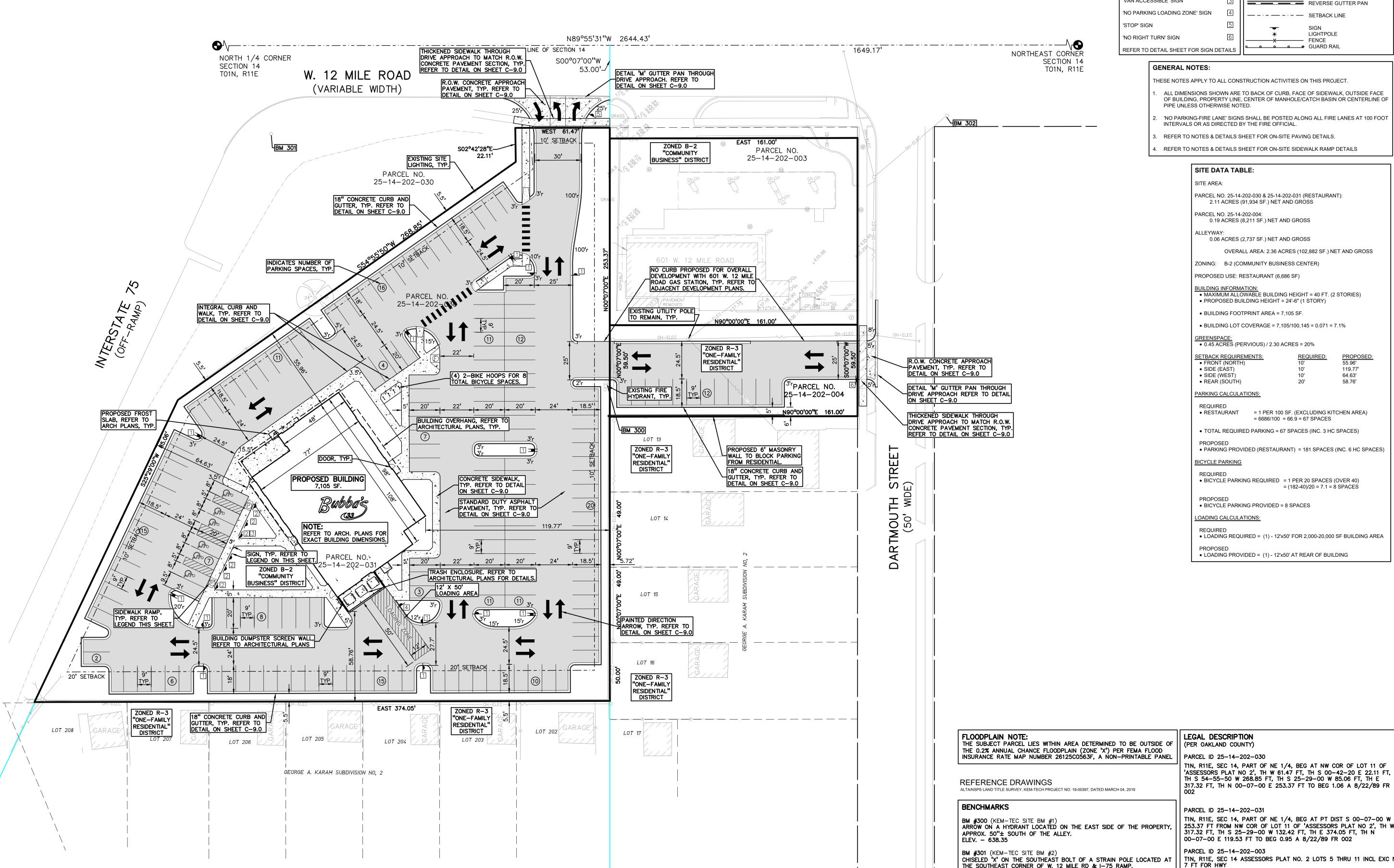
**SIDEWALK RAMP LEGEND:** LEGEND: CONCRETE PAVEMENT SIDEWALK RAMP 'TYPE P' REFER TO LATEST MDOT R-28 ASPHALT PAVEMENT STANDARD RAMP AND DETECTABLE WARNING DETAILS GRAVEL SIGN LEGEND: w w w WETLAND 'NO PARKING FIRE LANE' SIGN BARRIER FREE PARKING' SIGN CONCRETE CURB AND GUTTER 'VAN ACCESSIBLE' SIGN REVERSE GUTTER PAN
