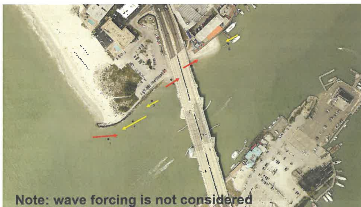
Figure 48. A concept model for the tidal flow pattern directly related to the sedimentation at the project site.
