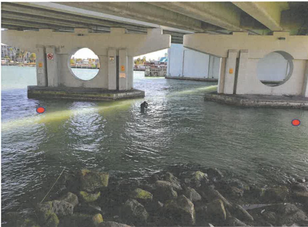
Figure 18. Short-term tidal current measurement at the project site.
