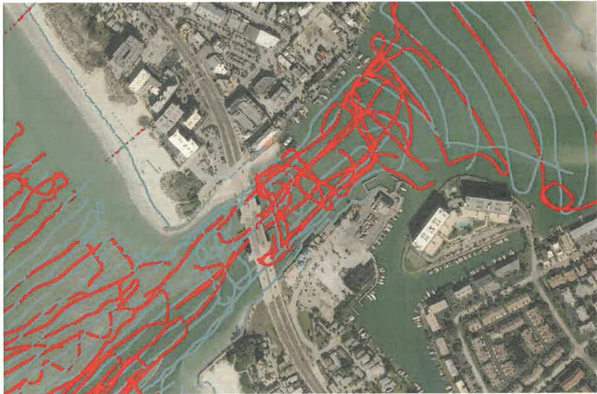
Figure 16. Coverage of the multi-beam bathymetry surveys conducted in 2018 and 2019.
