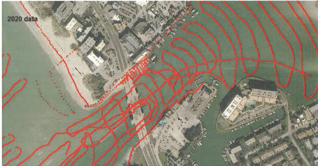
Figure 14. Coverage of the bathymetry survey conducted in June 2020.
