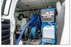
For carpet cleaning at these locations, AJI will be using a van equipped with a CDS 4.8 truck mounted, van-powered cleaning system from HydraMaster. These systems feature OverDrive™ Power Train Technology which allows us to deliver a deep clean to your facilities. The system is equipped with two solution outlets for dual wand capability, three speed settings and a 100 gallon recovery tank for uninterrupted cleaning.
