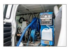
CDS 4.8 truck mounted, vanpowered cleaning system from HydraMaster.
