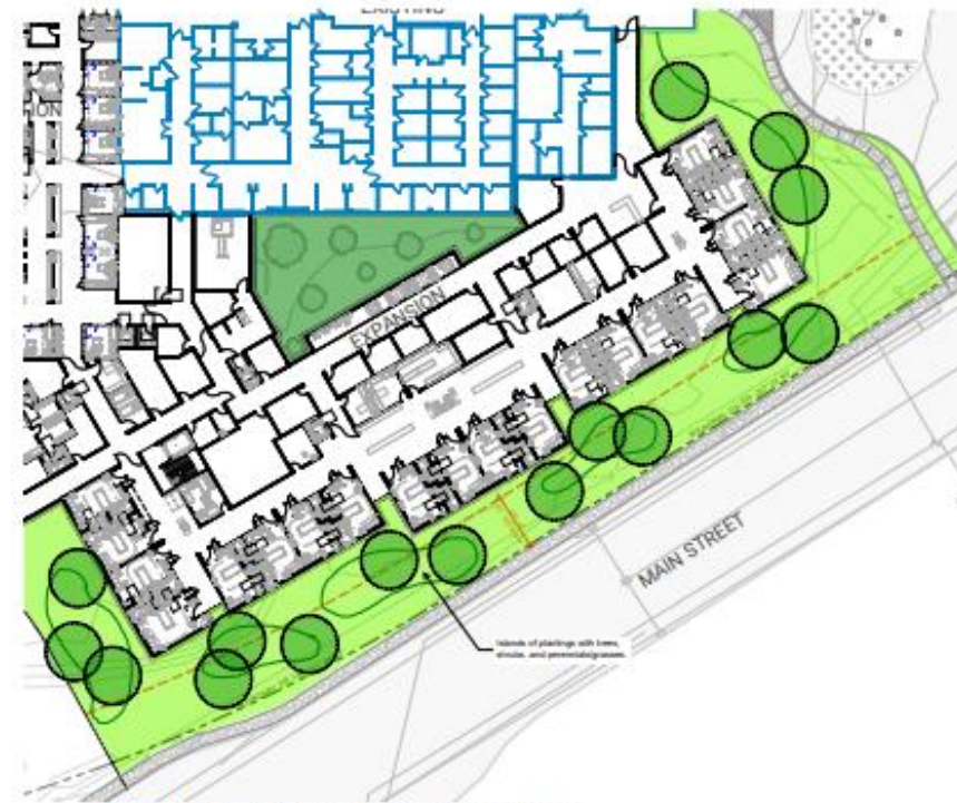
1 Alternate 1: Vault Option for Stormwater: Under building vault with frontage landscape bermed with lawn and trees, and islands of landscape.
