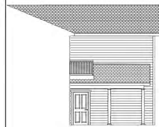
PORCH ELEVATION SCALE 3/16" = 1'-0"
