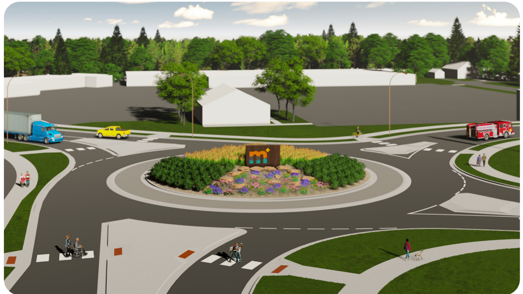
Visualization shows the roundabout design at Country Club Drive intersection, with potential landscaping of the roundabout center. The roundabout accommodates vehicles of all sizes, as well as people who walk, bike or roll.
