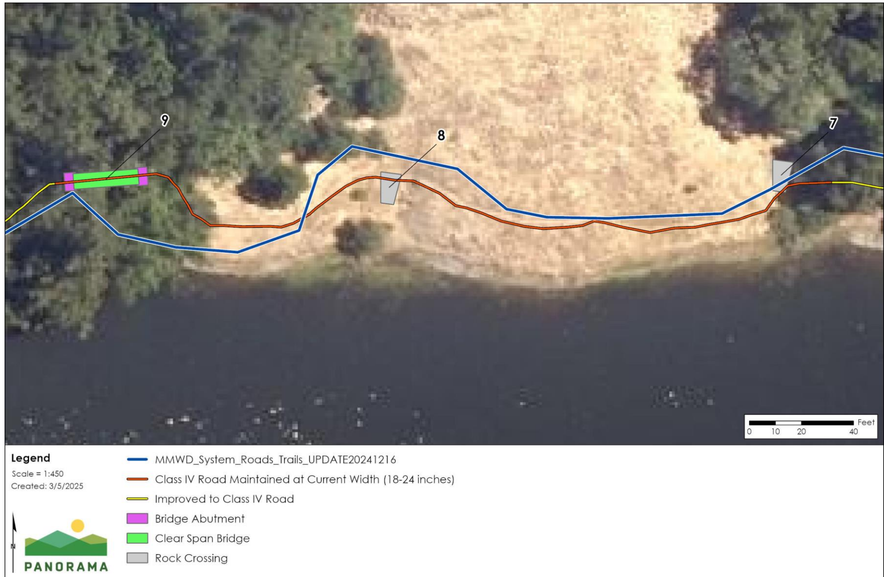
Figure 2 Liberty Gulch Road Revised Project From Stream Crossing Sites 7 to 9
