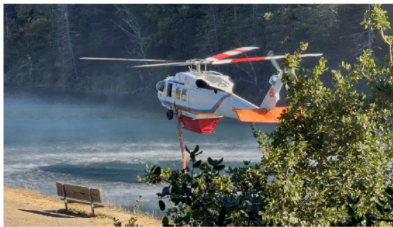
6PG uses its snorkel to refill its 1100-gallon tank at Phoenix Lake
