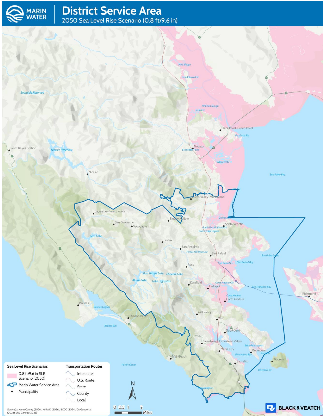
Figure 13-1. Area Inundated by a Sea Level Rise of 0.8-Foot
